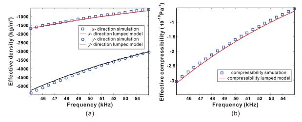
FIG. 3. Effective densities and compressibility extracted from full-wave simulations and predicted by the lumped model. (a) Effective densities in the *x* and *y* directions. (b) Effective compressibility. At 50 kHz, the desired density and compressibility are achieved.
