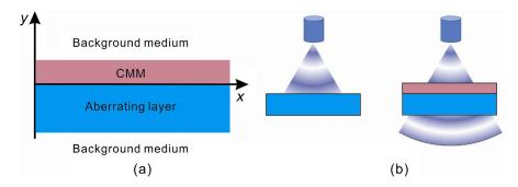
FIG. 1. (a) Schematic of the CMM, the aberrating layer, and the background medium. (b) Concept of the CMM for enhancing the sound transmission. The acoustic energy is blocked by the aberrating layer due to the large impedance mismatch (left), while it can transmit with high efficiency if placing the desired CMM adjacent to the aberrating layer (right).
